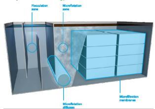
The microflotation process of the akvoFloat™
